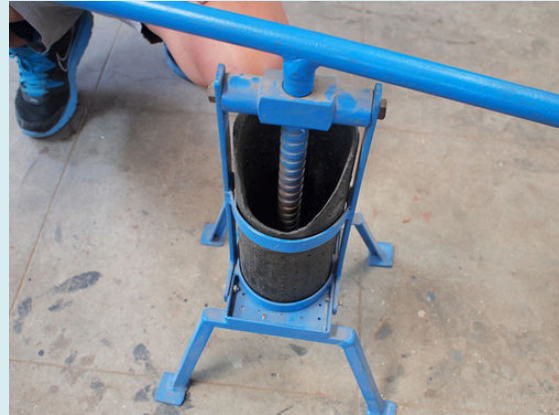
Figure 5: Screw press used to produce compressed coals.
