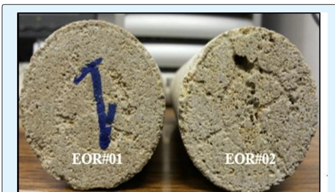
Figure 9: Wormholes created in the Low pH EDTA flooded Core (pH = 4.5; right core) compared to the High pH EDTA flooded one (pH = 12; left core).
