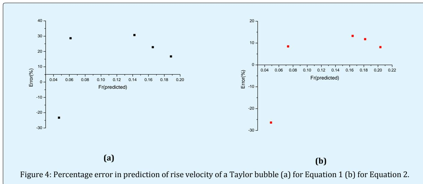
Figure 4: Percentage error in prediction of rise velocity of a Taylor bubble (a) for Equation 1 (b) for Equation 2.
