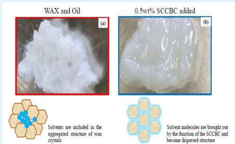
Figure 9: Out looks of the samples at 35°C. (a): Original WAX and Oil system, (b): 0.5wt% SCCBC added to original system. Lower illustrates are schematic image of each wax crystal and oil structure.
