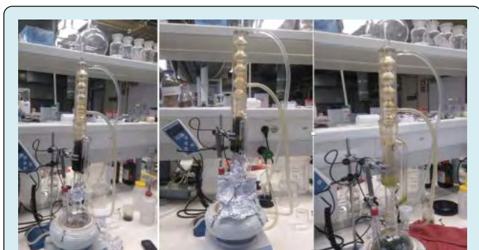
Figure 19: The stages of Microalgae Lipids extraction.
