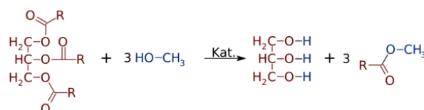
Figure 17: Generalized transesterification reaction [56].
