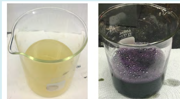
Figure 11: Left-7.5 wt% HCl and 7.5 wt% HEDTA acid-solution before the reaction; Right-effluent solution after reaction.
