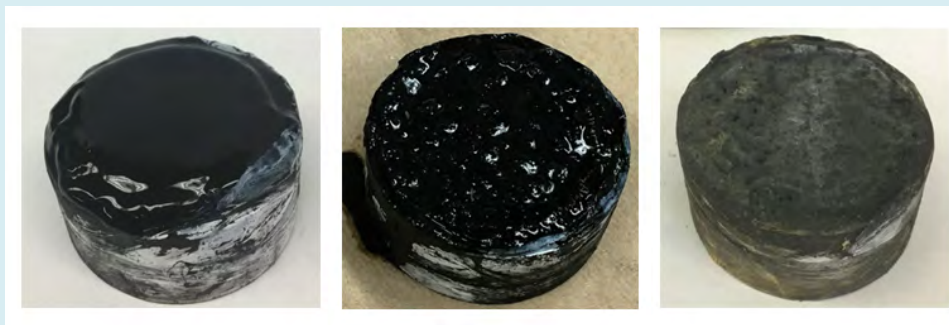
Figure 7: Left-filter cake after static filtration at 300 psi and 250°F; Middle-remaining filter cake after soaking for six hours with 7.5 wt% HCl at 300 psi and 250°F; Right-remaining filter cake after drying at 212°F for three hours.
