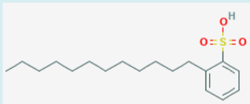
Figure 7: structure of dodecylbenzene sulfonic surfactant.
