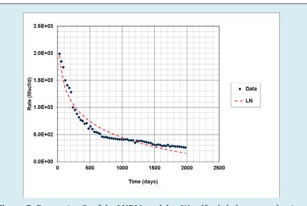
Figure 2: Regression fit of the LNDM model to Woodford shale gas production.
