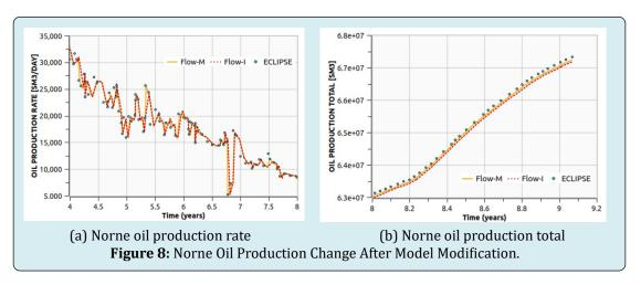
Figures 8(a) shows the modified simulator diverging from its unmodified counterpart at multiple different points during oil production. This is most noticeable at some points 4.3, 5.4 and 6.7 on the timescale. Thought these points don't all show an improved production rate, the change seems to be mostly positive. This is reflected in Figure 8(b) where we see that overall oil production is higher. It should be noted however, that the ECLIPSE simulator still shows higher production overall.
