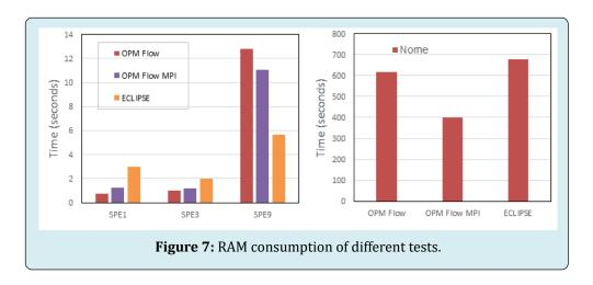
The RAM usage when running the SPE 9 tests was less for OPM Flow than that of Eclipse. However the Norne dataset showed significantly less RAM consumption when run on Eclipse. Using MPI drastically increases RAM consumption on OPM Flow, especially when running the Norne dataset.
