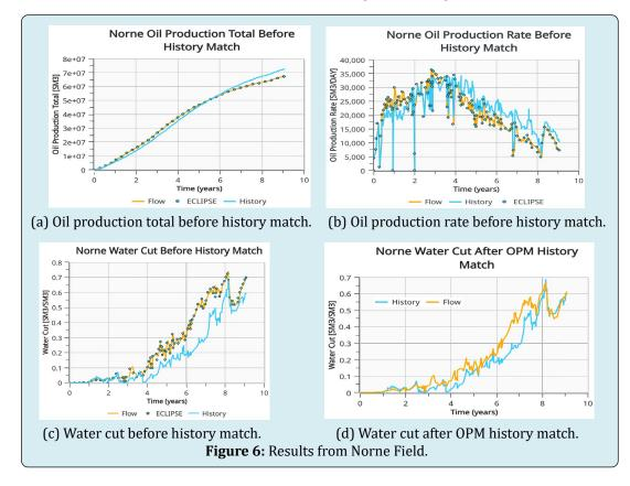
As can be seen in Figures 6, the simulators show near identical results with the Norne dataset. The base dataset however, does not give a good match with the actual production history of the reservoir. This base dataset under performs in every production metric shown. On the following page, the history matched values can be seen. As was stated in the limitations before, values for the Eclipse simulator were omitted due to an issue with oil-water relative permeability.
