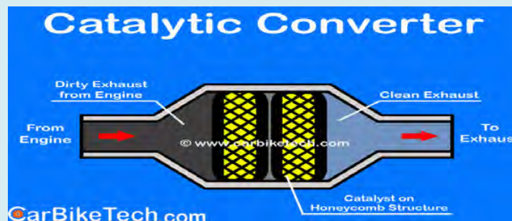
Figure 56: Typical configuration of the existing exhaust pipe line in internal combustion engines.
