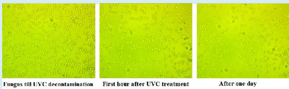
Figure 9: Decontamination with repacked fibers. The last two figures (central and right) represent the decontamination procedure with two types of packing fibers in the decontamination core. As it is observed after the 5 min of the UV-C radiation some colonies continue to remain in the fluid. This relates to the remaining large intervals between the fibers during the laminar flow of the yeast liquid.
