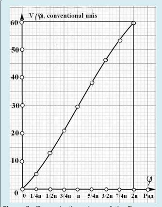
**Figure 3:** Change in the volume of the Torus space depending on the vortex angle  $\varphi$  .
