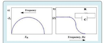
**Figure 2:** (a) Nyquist plot and (b) Bode plot for the simple equivalent circuit where resistor and capacitor in parallel [15].
